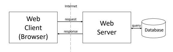
Figure 4.1: The client-server model on the web.
