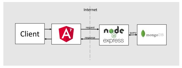
Figure 5.1: The overall architecture of TreeTest.
